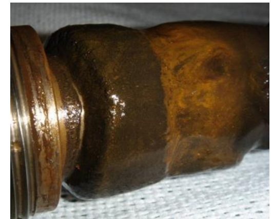
Typical WSC iron particles collected on magnetic filter rods
